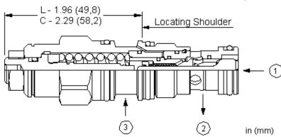
Counterbalance valves with pilot assist are meant to control an overrunning load. The check valve allows free flow from the directional valve (port 2) to the load (port 1) while a direct-acting, pilot-assisted relief valve controls flow from port 1 to port 2. Pilot assist at port 3 lowers the effective setting of the relief valve at a rate determined by the pilot ratio.
