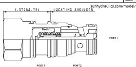
This valve is a pilot to open check valve. It has a sealed pilot, a steel seat, and is non-vented. It allows free flow from the valve (port 2) to the load (port 1) and blocks flow in the opposite direction. Pressure at the pilot (port 3) will open the valve from port 1 to port 2. Pilot pressure needed at port 3 to open the valve is directly proportional to the load pressure at port 1. Pressure at port 2 directly opposes pilot pressure.
