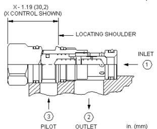
This valve is a spring biased closed, pilot-to-close check cartridge that has a 1.8:1 pilot ratio. The valve allows flow from port 1 to port 2 and blocks reverse flow. Pressure at the pilot port opposes pressure at port 1 at a ratio of 1.8:1. This valve is most often used in regeneration circuits.
