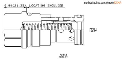
Free-flow, nose-to-side check valves are on/off circuit components that allow free flow from the inlet (port 1) to the outlet (port 2) and block flow in the opposite direction.
