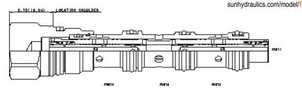
Synchronizing flow divider/combiners are sliding-spool, pressure-compensated devices used to split flow in one direction and combine flow in the opposite direction. With a sychronizing feature, these valves can be used to allow two hydraulic cylinders to fully stroke and synchronize at the end of the stroke. When the first cylinder has reached the end of its stroke, a pressure-compensated, reduced flow is metered to or from the second cylinder until it also reaches the end of its stroke.
